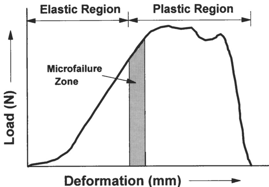
**FIGURE 1.** The load-deformation curve. It should be noted that the divisions illustrated in the graph represent a generalization. The microfailure zone is shown to begin at the end of the elastic region, but can occur before this point on the curve.
